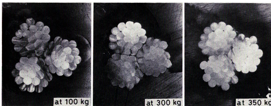
Fig. 3.39. Cross sections of 3-ply cord 19-yarn strand at various tensions.
