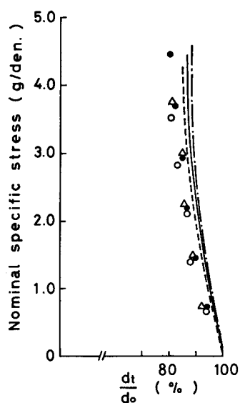
Fig. 3.45. Calculated and experimental values of diameter change by tensions of 2-ply cord 7-year strand at various surface helix angles, \Delta ; experimental, ----; calculated, for 25.1° surface helix angle, \bullet ; experimental, —; calculated, for 29.9° surface helix angle, \circ ; experimental, -.-.-; calculated, for 35.4° surface helix angle.
