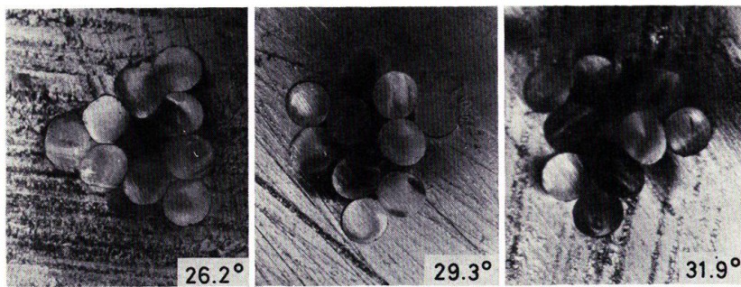
Fig. 3.32. Cross sections of 3-play cord 3-yarn strand at various surface helix angles.
